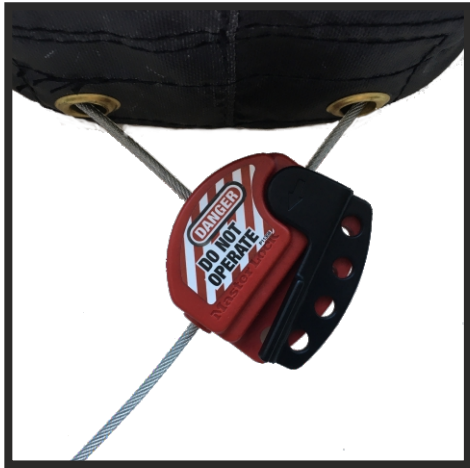
SECURE AND LOCK THE ENTRY WITH A MASTERLOCK CABLE LOCKOUT
